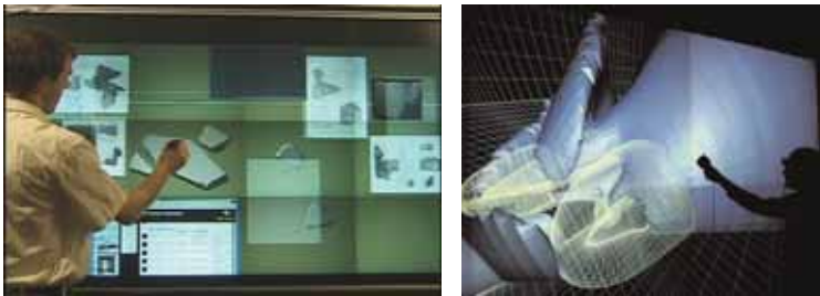
Figure 4.15: Left: Stanford Interactive Mural. Photo courtesy of HCI Group, Stanford University. Right: Display Wall at UC Davis VR Lab. Photo courtesy of Oliver Staadt, UC Davis and University of Rostock. Both tiled screens have visible tiling artifacts.
