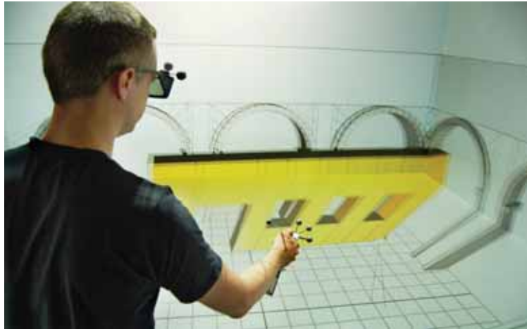
Figure 6.55: Generative modeling of walls. The user aims with the joystick at the small green sphere, resizing the wall by dragging. Note that for the user, the black line visible on the floor appears to start at the joystick position.
