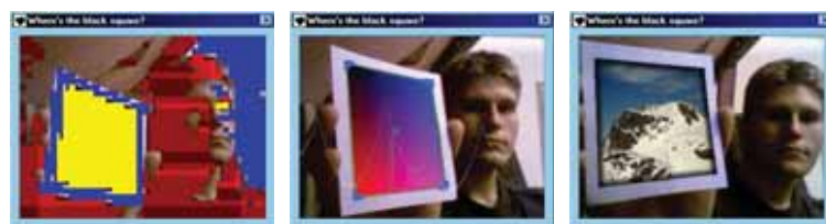
Figure 3.28: Own implementation of a 2D AR marker application. Marker identification (left), corner detection (center) and compositing of a respectively warped photo on the marker (right).
