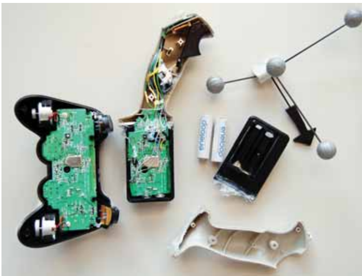
Figure 2.54: The electronics of a gamepad (left) are cut and integrated into a joystick grip (center), with a battery compartment on the bottom.
