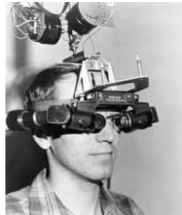
Figure 2.4: The Sword of Damocles , the first HMD to show computer generated content, by Sutherland in 1968 [Sut68].
