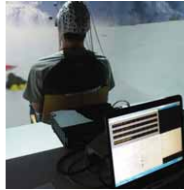
Figure 5.4: Brain computer interface (BCI) used as input to control navigation in the DAVE. A state change is detected within about two seconds and send to the DAVE server via UDP or TCP. See section 6.3.10.1 for a description of the applications.
