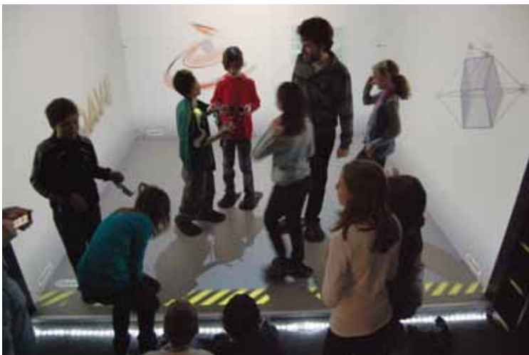
Figure 6.85: We have a step that is also marked by black yellow stripes. Later we added a room light in form of an LED strip. This enables basic orientation in the DAVE even when the projectors show black, while it does not influence projection contrast or the tracking system notably.
