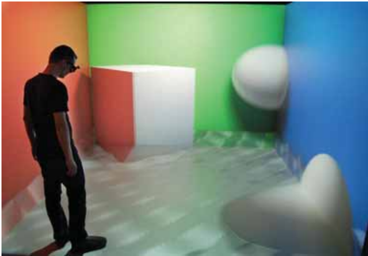
Figure 6.61: A pathtracer implemented with CUDA, ported to the DAVE with the Davelib. Note the color bleeding, especially visible at the left side of the box. To achieve a high enough framerate, the quality is low and a lot of noise is visible, that this photo does not show as the camera exposed over a few frames.
