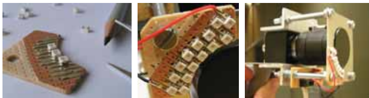
Figure 2.41: Infrared illumination with SMD LEDs. In addition to the housing on the right, an IR filter is attached in front of the lens to filter out visible light.
