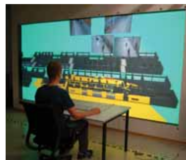
Figure 6.27: AUTOVISTA: A CCTV surveillance system with a 3D model to provide spatial context.
