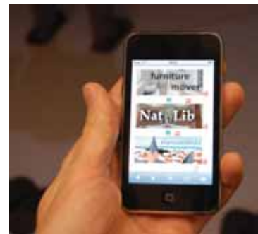
Figure 2.26: An ipod touch is used for system control, realized with a web browser.
