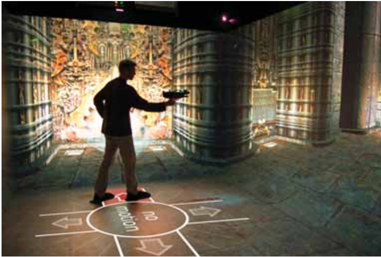
Figure 5.2: In this Quake III arena game, the absolute position of the user is employed to control the walking speed. It turned out that this method is rather hard to use. The arrows were added for illustrative purposes. Also note that the photo was taken in mono, from a point of view near the camera and the user does not wear the glasses, for a nicer photo.
