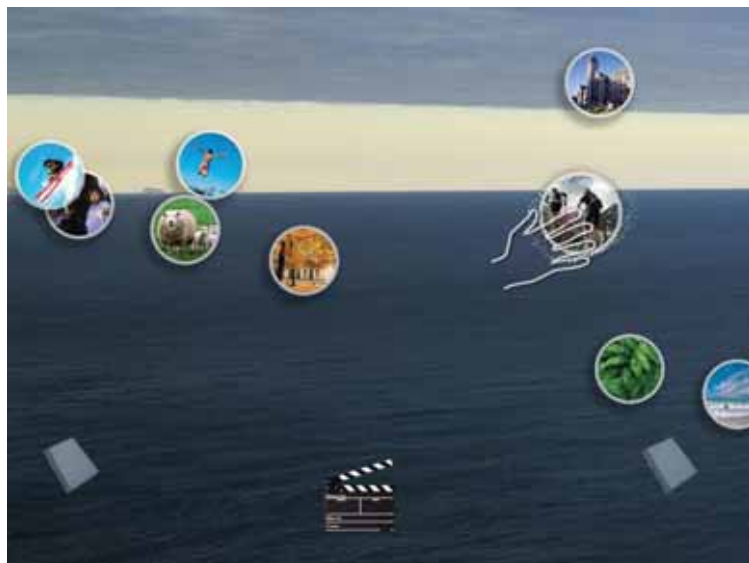
Figure 6.2: Screenshot in idle mode. When nobody touches for some 10 seconds, an animation of a moving hand indicates how and where to drag the icons. The icons move from left to right on curved paths, thereby moving up and down. They have inertia and can be flicked across the screens. Background images changed from time to time, professional media was shown with video clips or slide shows, depending on the tool the icon is dragged to. Image courtesy of HIT Lab NZ, University of Canterbury.
