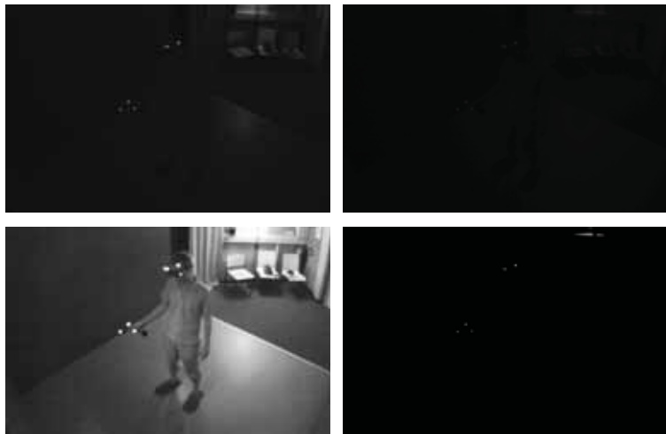
Figure 3.4: An exemplary camera image (top left, enhanced levels in the bottom left) with some ambient light present. The result of filtering and thresholding is shown in the top right (enhanced levels in the bottom right). One marker of the glasses is not recognized. The ambient light leads to five additional detections which does not break or significantly slow down the tracking of the glasses and the joystick.
