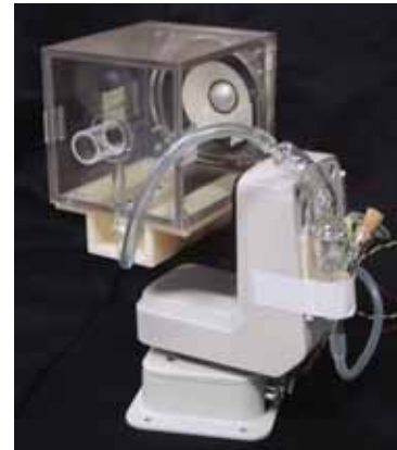
Figure 2.12: Olfactory device with nose tracking. Photo courtesy of [YKNT03].
