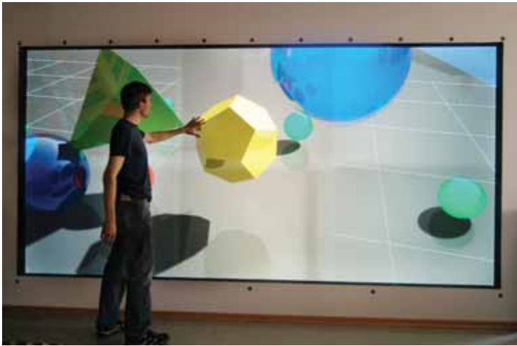
Figure 6.30: A simple realtime raytracer on the HEyeWall, here still with a few clipping artefacts due to the calibration matrix.
