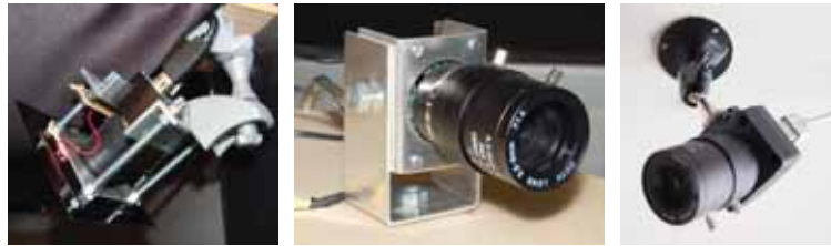
Figure 2.56: The camera mounts in the DAVE are hard to adjust (left). Custom camera mounts for the HEyeWall work much better (center). A cheap and good option is shown on the right.
