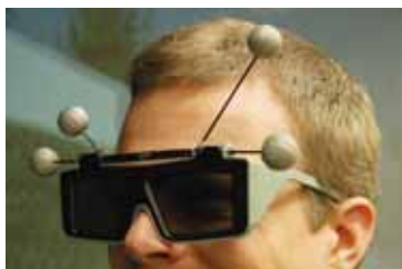
Figure 2.30: Lightweight shutter glasses with retroreflective markers for head tracking.
